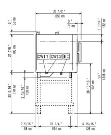
CWII Cold Water inlet 1 (cleaning) Cold Water Inlet 2 (steam CWI2 generator)
